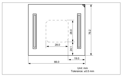
Figure 7 Dimensions for User System Interface Cable Head
